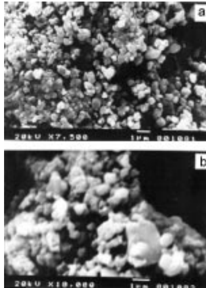
Fig. 2 SEM micrographs of the original microcomposite observed at different magnifications: a – \times 7\,500 ; b – \times 10\,000
